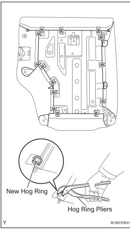
(b) Using hog ring pliers, install 14 new hog rings.
